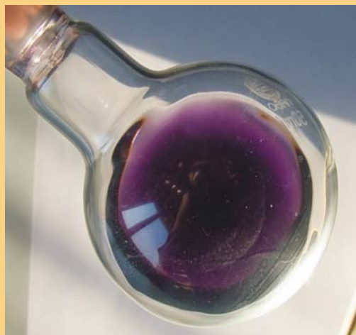
Hexane solution of carbosilane dendrimer Filled by cobalt oxide(II)
